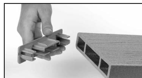
Do not block drainage hole. Make sure the drainage part of the end cap is on the bottom.
